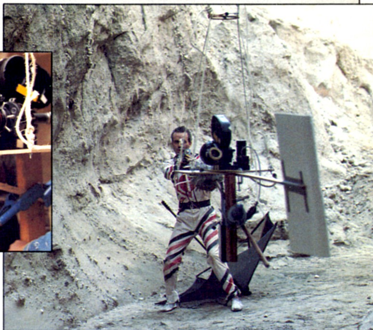
Filming Lars (David Clennon) in his battle with an alien "flying fish" (inset) using a camera rig designed by Robert Augur and Jim Zarlengo to give a bird's-eye-view of the attack. The tail rudder was added to give the Arri S camera in use a smooth flight.
